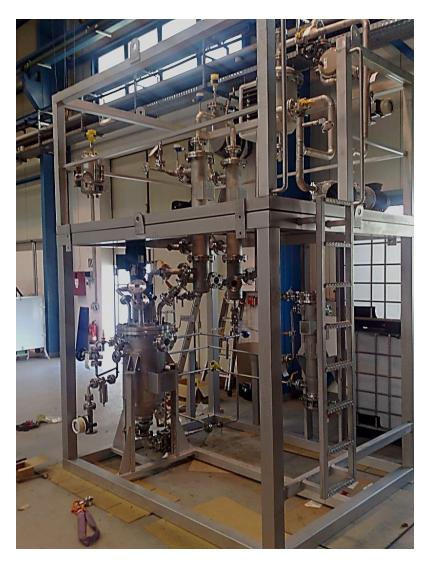
with hight temperature TO unit, with gas circuit for drying, with vacuum pump up to 1 mbar and with filtration system for heterogenous catalyst reactions
