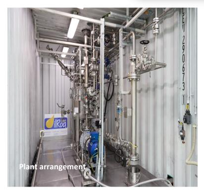
The test facility has a loop reactor with post-filtration unit, which make it possible to carry out different types of oleochemical and chemical processes such as :
